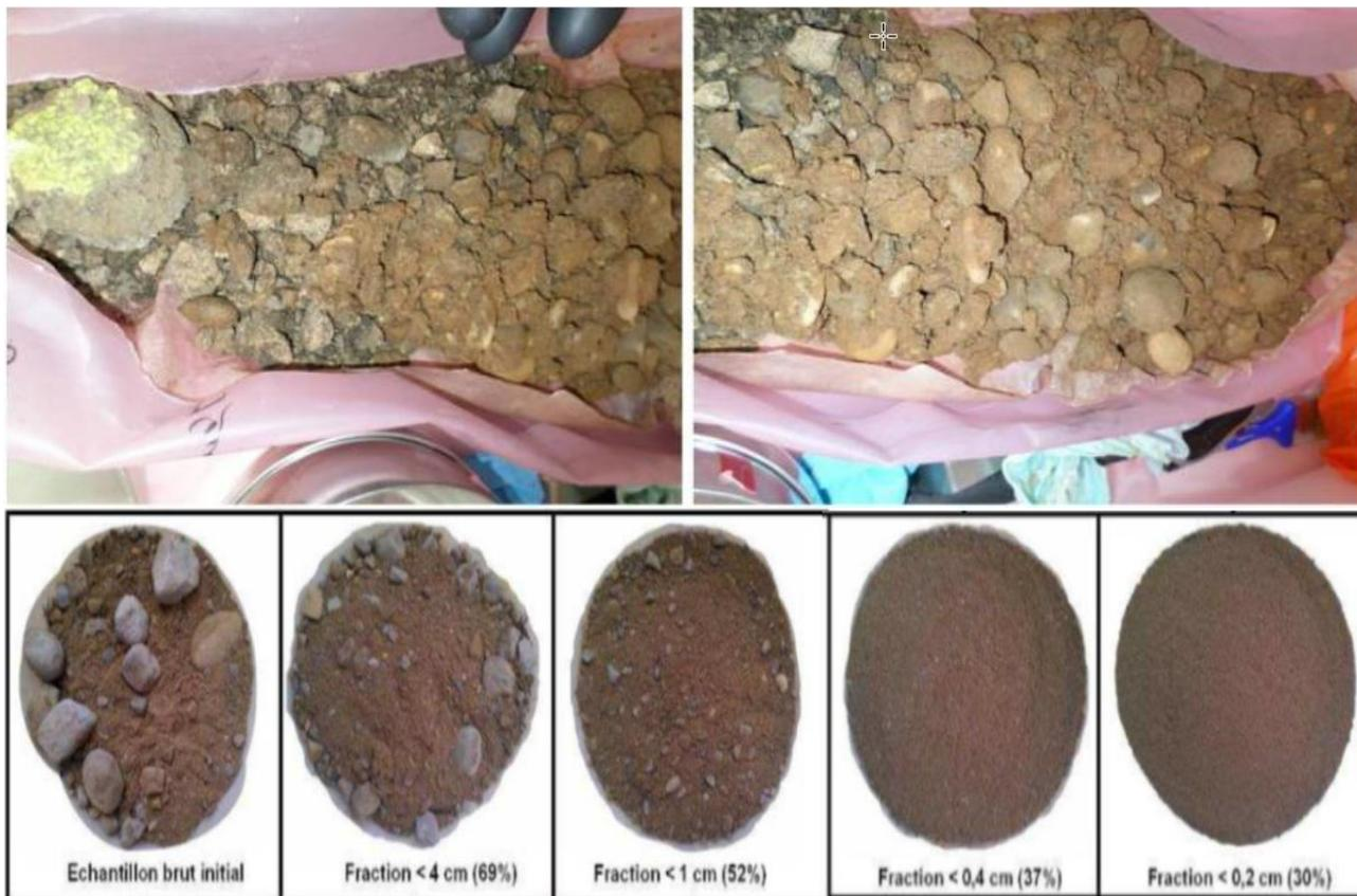
**Figure 5: Raw drilling core (top) and result of size segregation (bottom).**
