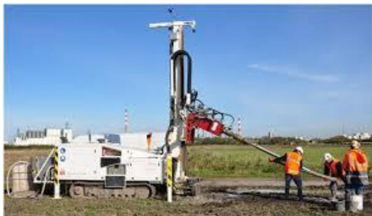
**Figure 3: Sonic drilling machine similar to the one used on UC3.**
